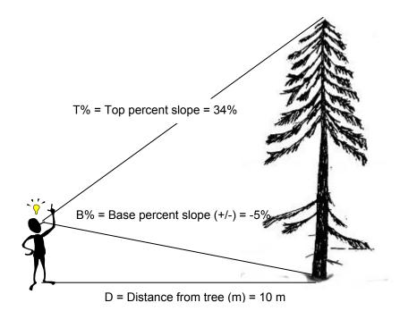
Figure 3. Tree height equals: Height (m) = D x (T% - B%). If the base percent is negative (reading eye-level to tree or on slope above tree DBH), then add B%, if base percent is positive (on slope below tree DBH) then subtract B%. Ht =  $20m \times (0.34 + 0.05) = 7.8 m$
